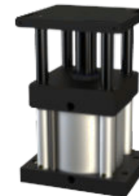
Lifter 4 Post. Ex: 5" bore, 4" stroke, main rod 1.75" dia and the 4 post at 1" dia. The post are guarded by thin wall tubing.
